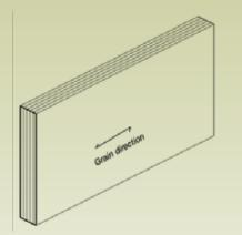
The biggest advantage of LVL is the fact that it is manufactured continuously, meaning it is available in almost any length. LVL - a high-strength engineered wood productwith an unlimited range of design and building applications
