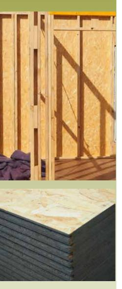
OSB has similar properties to plywood, yet is generally more cost-effective to manufacture, it can also be similar to, but stronger than particleboard.
