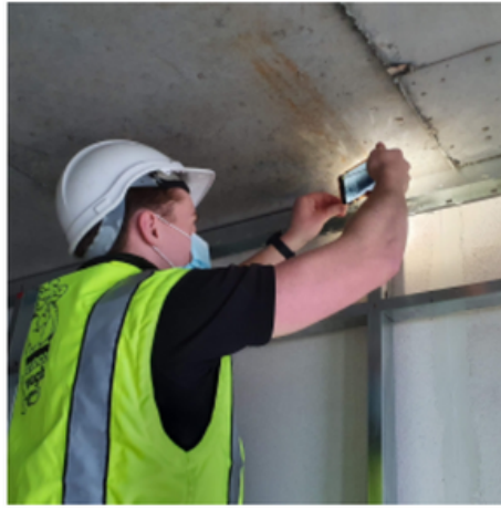
Studco site testing - investigating the Vortex track's response to uneven concrete slabs.
