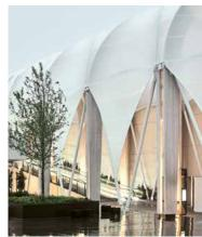
tarting from the arched glass roof of the Shopping Centre, we have designed a 110-metre long, arched passageway, which is based on a diagrid structure made from Italian larch glulam and topped with a stretch-resistant, semitranslucent PTFE canopy. Despite the openings in the edges of the structure, provided for cross ventilation, the design is extremely robust", describe the architects of "Make Architects" their Chadstone Link.
