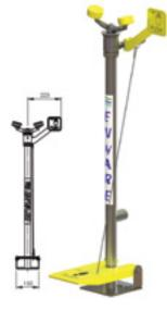
To meet AS4775 and ANSI Z358.1 performance requirements Enware Eye/Face Washes require: Minimum flow rate of 26 lpm (6.9 US gpm) at a dynamic pressure of 210 kPa (30 psi).
