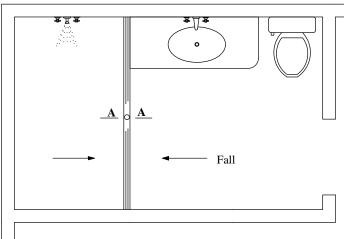
Seal with flexible caulking from the side wall of the 65I40-1200 to the underside of the tile.
