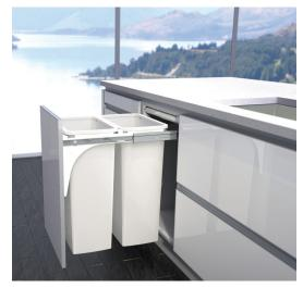
Four U-shaped air vents have been designed into the lip of the bucket, allowing trapped air to escape as the bag is pushed into the bucket cavity. This eliminates the frustration of trapped air restricting the liner, maximising bag volume.
