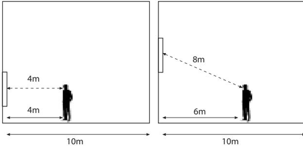
*Raising the screen elevation changes the viewing angle and viewing distance. It also pushes the viewer back a little to obtain a more comfortable view.*
