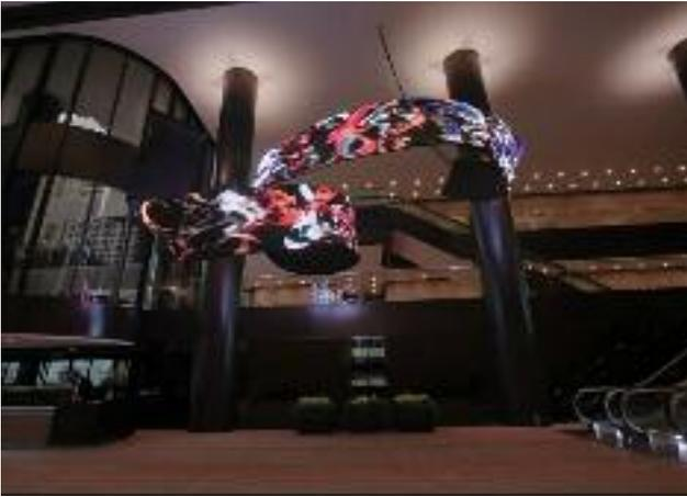
LED displays with 2 way flexibility not only allow the realisation of smoothly produced, uniformly curved shapes like canisters or circles, but can also twist to helical shapes. This opens up many more possibilities for a designer to be creative.
