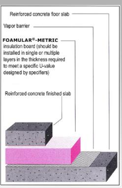
Recommended Material: FM 300/350, 75&100 mm (Common spec, 2 layers of FM 350/75mm) For Technical Information, Contact Mike Nagle - 0417 268 660 <u>mnagle@austech.com.au</u> • <u>www.austech.com.au</u>
