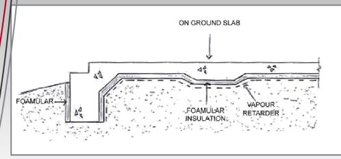
As Foamular is not affected by moisture, soil borne bacteria or mould it can be back filled against for gardens etc. with no loss of thermal a physical properties.
