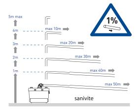
Increase size of horizontal run by one pipe size after 10m
