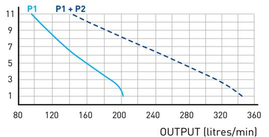
Example: Pump P1 is operating normally. It discharges 160 L/min at a pumping height of 5m. If pump P1 shows any signs of weakness or if the waste water inflow is too great, pump P2 starts up. The output is then increased to about 275 L/min, until the situation returns to normal.
