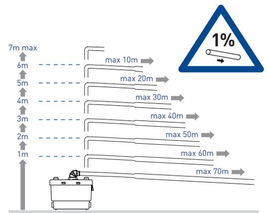
Increase size of horizontal run by one pipe size after 10m
