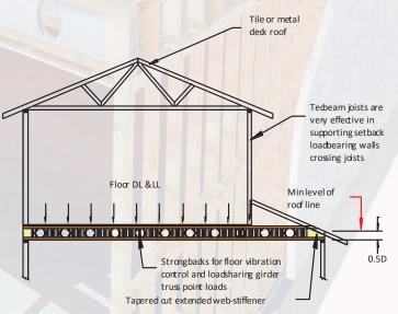
Tecbeam joists spanning to outside supporting wall
