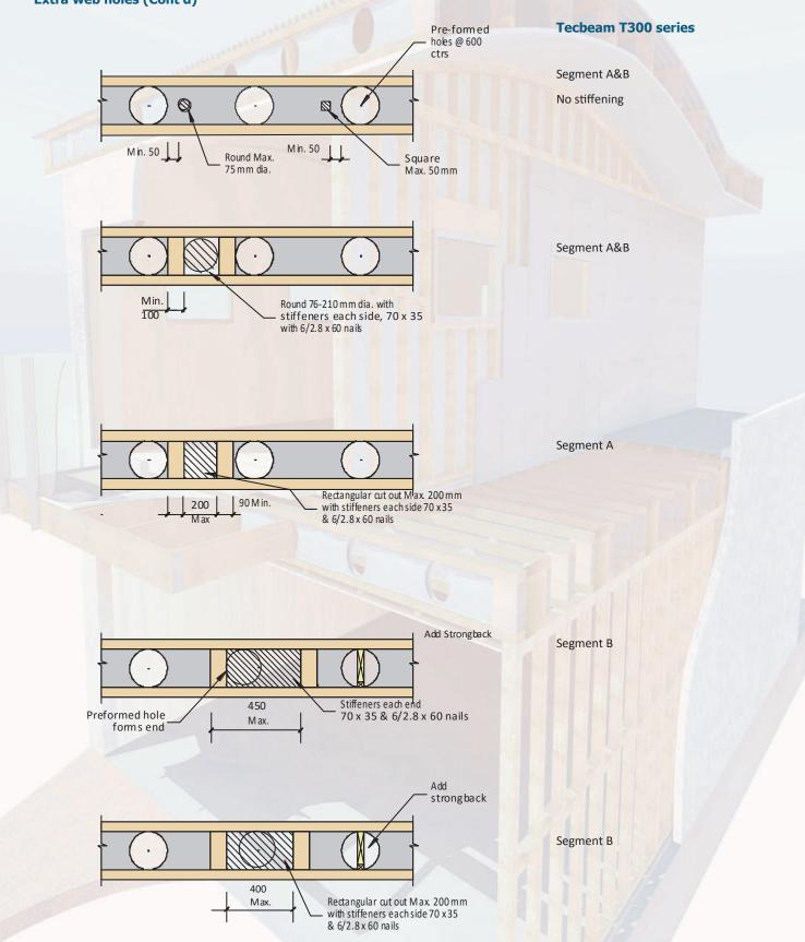
For T36 and T40 series, setback LBWs, continuous spans, and higher floor loading, refer to Tilling Timber Pty Ltd , Tecbeam Australasia or a structural engineer.
