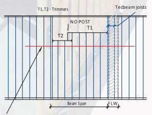
Beam concealed in Tecbeam web holes, continue paststair void for load sharing. For longer spans or higher loading, a steel section will be required.
