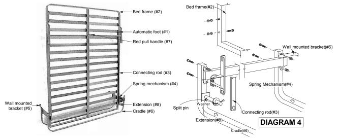
\* Attach the red handle supplied to the Automatic foot (#1) using the screws provided. To avoid damage to the connecting rod, be sure that the bed is lowered using the red handle.
