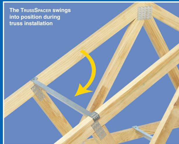
Not only does the TRUSSPACER position trusses accurately, but it has been designed to meet the requirements of AS4440-2004, the code for 'Installation of Nail Plated Timber Trusses' as a temporary truss chord tie<sup>1</sup>. This ease of operation means the TRUSSPACER can actually speed up roof construction and improve on-site safety for truss installers.
