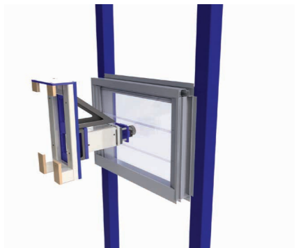
Load test in closed position
