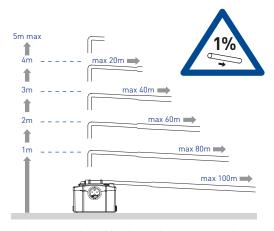
Increase size of horizontal run by one pipe size after 10m
