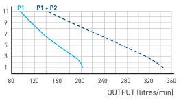
Example: Pump P1 is operating normally. It discharges 160 L/min at a pumping height of 5m. If pump P1 shows any signs of weakness or if the waste water inflow is too great, pump P2 starts up. The output is then increased to about 275 L/min, until the situation returns to normal.
