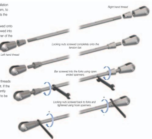
Each fork is supplied with a locking nut and pin to enable fixing to a connecting plate or anchor disc. The installation requires a twin-pin driver. Two driver bits of the appropriate size are supplied with each Ancon system. This type of fixing, known as 'Snake Eyes'\*, allows a high torque to be achieved without damage to the pin.
