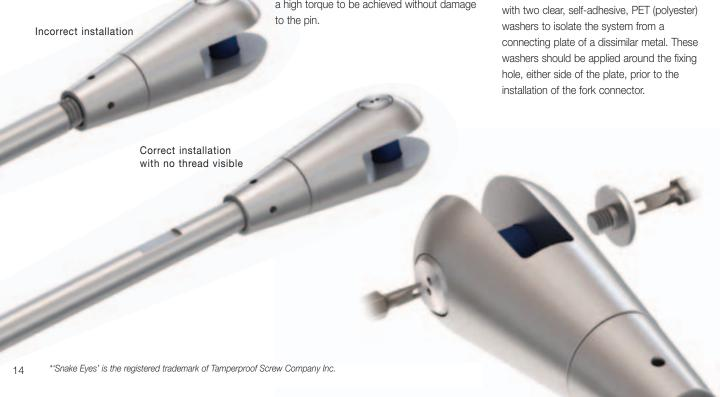
Forks must be correctly aligned, and positioned in the same plane to ensure that bending is not introduced into the tension system.
