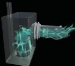
When the toilet is flushed the water level rises and the Saniflo pump operates automatically.
