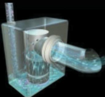
The resultant slurry is pumped out via the impeller on the bottom of the motor, through a pipe of just 20-25 mm in diameter, then stops automatically.
