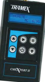
are mounted on the base which, during operation, transmit a low-frequency signal into the concrete floor. To carry out moisture tests simply brush any dust from a smooth area of concrete and also from electrodes, switch on the CMEXpertii and press to the surface to read the percentage moisture content.
