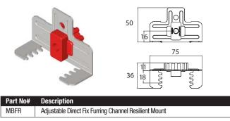
Resilmount MBFR can be used in wall applications with with Studco M308 16mm furring channel and  $\,$  M29 28mm furring channel.
