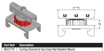
Resilmount M237TR can be used in ceiling applications to isolate airborne sound. Use this mount as the isolated coupling between the Studco M27 25mm Top Cross Rail and the Studco M29 28mm furring channel.
