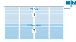
that all blades in the top halves of all the bays form a bank and operate simultaneously and all the blades in the lower halves of all the bays form a second bank and operate simultaneously. However, various switching and wiring configurations allow multiple windows to be controlled simultaneously or independently depending on individual preferences.
