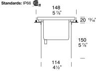
> Fluorescent Canister (PVC) (Supplied with Luminaire)
