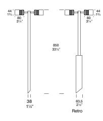
Accessories: Cable Joint Kit #CJK150 Frosted Lens #LENSEURF, RETRO 120/240 volt transformer /R (changes the luminaire to an IP56 rating).
