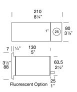
Fluorescent Canister (PVC) (Supplied with Luminaire)
