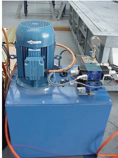
Hydraulic Power Plant
