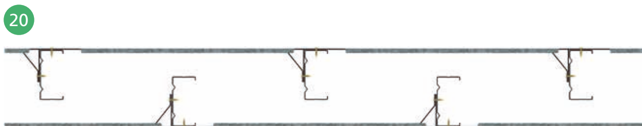
■ PLAN VIEW OF STAGGERED STUD FRAMING WITH FAST-FIX NOGGING INSTALLED BOTH SIDES
