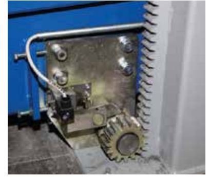
A steel safety gear, electrically interlocked rests on the internal toothed pinion which will lock the platform in the event of sudden release of the button or movement.
