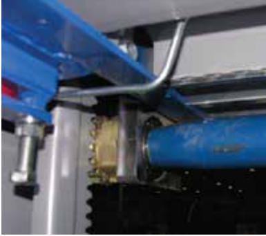
A hydraulically operated mechanical block located at the top of the column ensures platform safety at all times.
