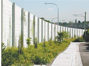
SoundBarrier panels are steel reinforced Hebel Autoclaved Aerated concrete (AAC), a solid masonry product that is very strong yet 25% the weight of standard masonry and quick to install.
