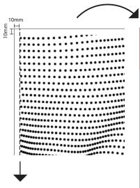
Dashed trim line for trimming of panel to pattern match edge to edge.
