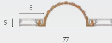
IS9055 Finger Guard Seal - hinge position
