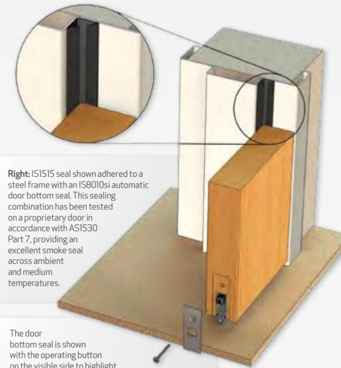
**Right:** IS1515 seal shown adhered to a steel frame with an IS8010si automatic door bottom seal. This sealing combination has been tested on a proprietary door in accordance with AS1530 Part 7, providing an excellent smoke seal across ambient and medium temperatures.
