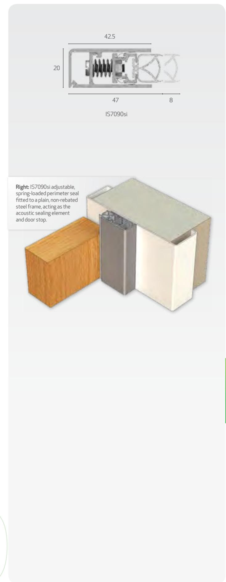
**Right:** IS7090si adjustable, spring-loaded perimeter seal fitted to a plain, non-rebated steel frame, acting as the acoustic sealing element and door stop.
