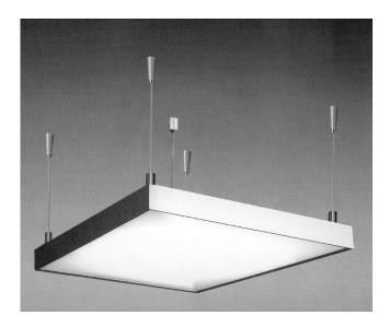
**High Output LED** Pendant light panel, the main body is manufactured from die cast aluminium with ultra pure aluminium. Supplied as standard with opal diffuser panel. The LED driver is remote mounted in the ceiling cavity. Using new generation Led the pendant has  $430 \times 0.2 \text{w}$  LEDs. Supplied in silver powder coated paint finish. Suspension length 1 metre
