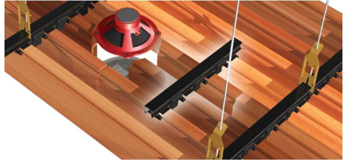
5. Ensure that any smaller joints are properly supported with a short TCR rail and clips covering the adjacent profiles.
