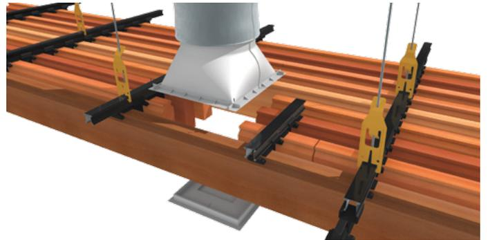
6. Austratus has a natural acoustic rating, which can be further enhanced to suit various application requirements, with the addition of acoustic insulation. Simply cut the insulation to the required shape and size, then lay it on top of the timber profiles. Technical information is available on request.
