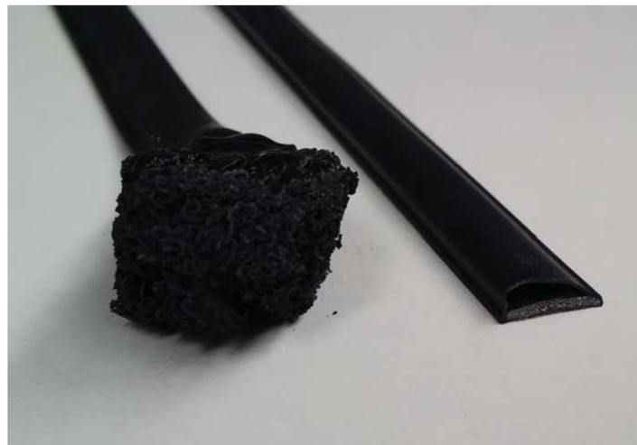
*Right image: shows LAS1602BB seal before and after exposure to elevated temperature*
