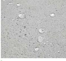
This concrete surface was sealed with a penetrating sealer, making it resistant to liquids.
