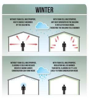
In winter, cold, uninsulated metal walls quickly remove any heat generated in a building. Foam Cell MULTIPURPOSE will reduce this heat transfer and help make the building feel warmer. It will also reduce the risk of condensation by providing an insulating layer between potentially warm, moist air and the cold metal.
