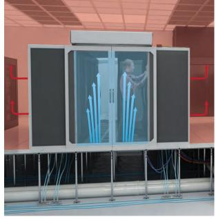
SmartAire P monitors the static pressure differential from the contained cold aisle to the hot aisle in order to maintain a balance when rack loads vary. This balance reduces bypass airflow through servers, racks and other containment structures.
