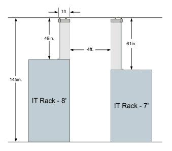
Note: Although you may choose any combination of track lengths to add up to your total horizontal row length, it is recommended you use the minimal number of track lengths possible to reduce costs, improve ease of installation and reduce potential air leakage at each seam. It is important to ensure that the overall partition track length is greater than or equal to the total row length measured.
