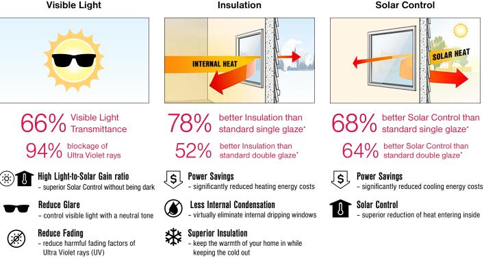
\*Note: Data using centre of glass performance in NFRC standards and using 6mm clear float single glaze, 6/12/6 clear float double glazed unit with air gap and 6/12/6 Insulglass LowE Max<sup>®</sup> double glazed unit with argon gas and coating to surface #2.
