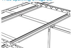
The deep Omega Bar has a maximum spanning ability of 2000mm. The wide spanning bar requires 25% less primary channels, top fixings and brackets, saving installation time and materials.
