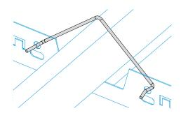
In areas where it is necessary to restrict access to the ceiling void, System 150 offers a security clips that holds the tiles into the supporting grid. This is ideal for airports and other security driven environments, including schools and lavatories.
