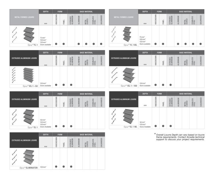
Where a project requires a reasonable level of rain defence this system remains suitable and offers an additional weather-lip system (WL) to reduce water penetration. This system is the most commonly used and specified system incorporated in Commercial and Industrial applications including hospitals, apartment buildings, carparks, high rise buildings, water processing plants, mining workshops and industrial warehouses.
