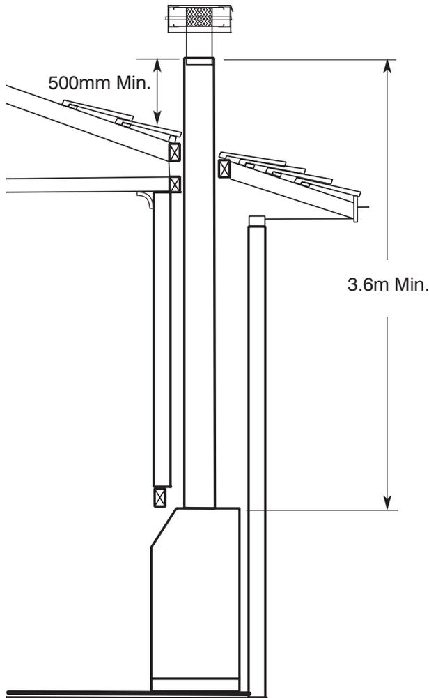
A minimum of 3.6m flue is required to protrude 500mm above roof line.
