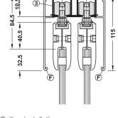
Ceiling installation Ceiling installation with running track with double running track and 2 x clip panel for integration in and clip panel 115 mm suspended ceilings
