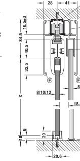
Ceiling installation with running track and clip panel 115 mm including fixed component on wooden supports (wet sealed) provided on site
