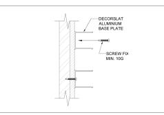
O6 Attach the second piece of tracking plate and use spacers in between, repeat until all tracking is spaced to the surface.
