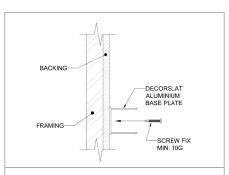
05 Attach the first piece of backing plate to the surface
