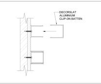
08 Attach the second piece of Clip-On battens, repeat until all battens are in place.
