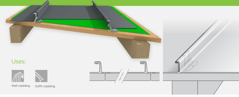
Single lock standing seam profile and installation shown on 17mm ply board over supports.
