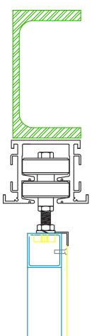
Multi Direction Track And Rollers for screens that can turn and stack in various locations.
