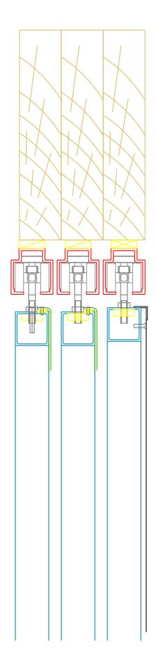
Linear track allow side by side track installation where screens move in two directions, independant of each other.
