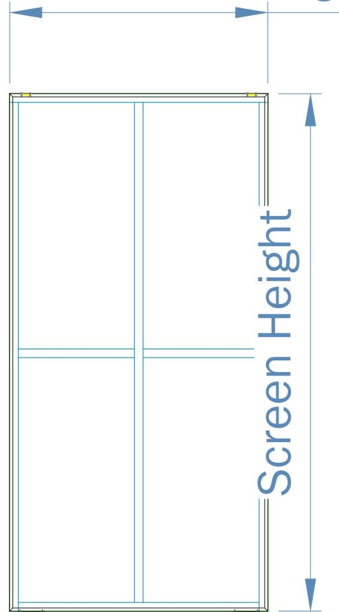
Screens are manufactured using aluminium welded frames.
