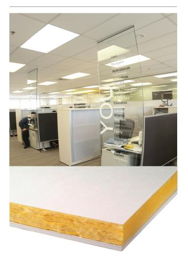
Sound absorption rating:  $\alpha^w$  1.00 - Class A (AS ISO 11654); NRC 0.95 / SAA 0.95 (ASTM C423); Type E-200 mounting (ASTM E795); University of Auckland Test Report T0516-10
