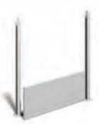
Concrete posts into the ground & push the first lower panel into place.
