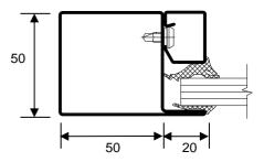
Standard profile with rubber beading (internal application)
