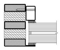
Standard profile with silicone beading (internal or external application)
