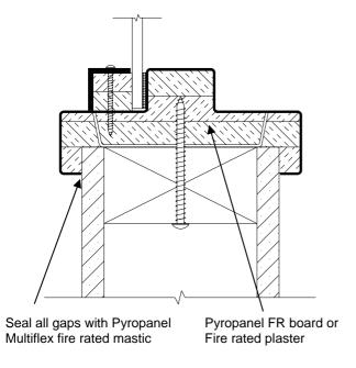
Typical wall fixing for masonry and pre-cast concrete walls
