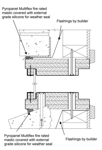
Ensure all gaps are tightly sealed with fire rated sealant, and that the frames are fully packed with Pyropanel FR board, Fire rated plaster, mortar or concrete. Back of window frame must abut fire rated element of wall (generally brick).
