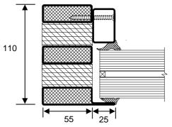
Standard profile with rubber beading (internal application)
