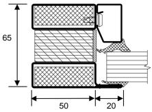
Standard profile with rubber beading (internal application)
