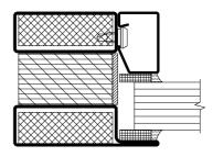
Standard profile with silicone beading (internal or external application)
