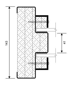
Pressed metal single rebated window frame with double glazing
