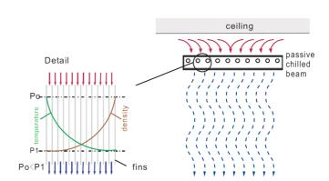
Figure 3: Passive Chilled Beam Natural Convection
