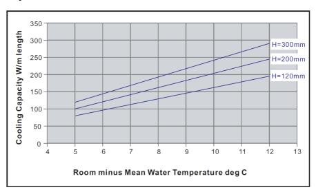
Figure 8: Cooling capacity model 300
