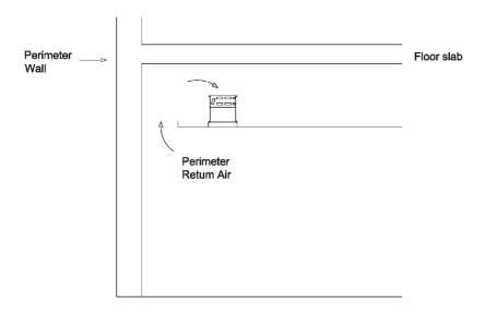
Figure 5: Air path for return air
