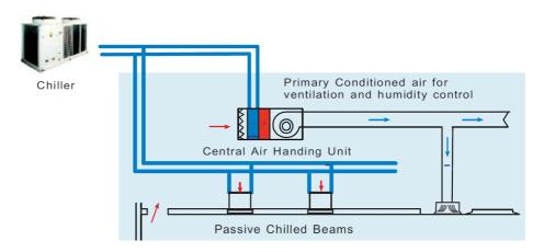
Figure 2: Passive Chilled Beam System
