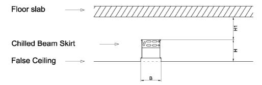
Figure 6: Free space above the chilled beam
