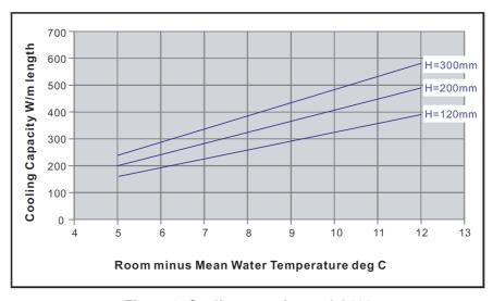
Figure 9: Cooling capacity model 600
