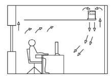
Figure 4: Positioning passive chilled beams
