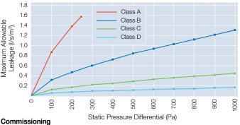
The test pressure should not exceed the design pressure to which ductwork from The *Kingspan* **Kool**Duct® System has been fabricated. When pressure or air-leakage testing is known to be necessary, ductwork should be fabricated to withstand the test pressure, if greater than the design pressure.
