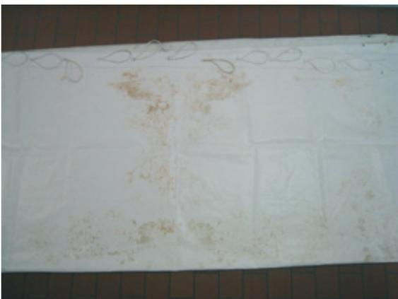
Example of moulding for wrongly stored temporary structures. It is clearly to see that mould has formed at the internal part of the folded material, probably due to the fact that the material was stored wet or that the storage place was not adequately dry.
