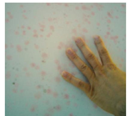
Fabric under fungal attack. Micro organisms have already invaded the coating with possible deteriorating of the original material characteristics.
