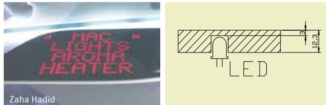
To obtain a more diffuse effect, the light source is generally installed at a distance (typically 15 cm) from the back of the panel. The routing can be done with a CNC machine in any kind of pattern or design. Playing with varied depths of the routed pattern and creating a 3D relief gives the possibility to create an effect reminiscent of a painting.
