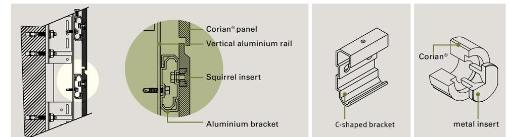
Overlapped or open joints are located on all panel edges. The joint width depends on the thermal expansion coefficient of Corian® and the panel dimensions. The minimum horizontal width is 16 mm, and the minimum vertical width is 8 mm.
