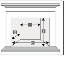
\*\* If using the GreenStart Igniter the opening width required is a minimum 915mm at the front of the opening for the first 90mm depth. Always refer to the relevant installation manual to confirm clearances available at www.lopi.com.au
