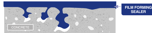
DIAGRAM DEPICTING CLOSE UP OF CONCRETE SURFACE USING A FILM FORMING SEALER
